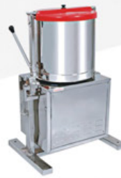
TILTING TYPE WET GRINDER (10, 15, 20, 40 Ltrs)
